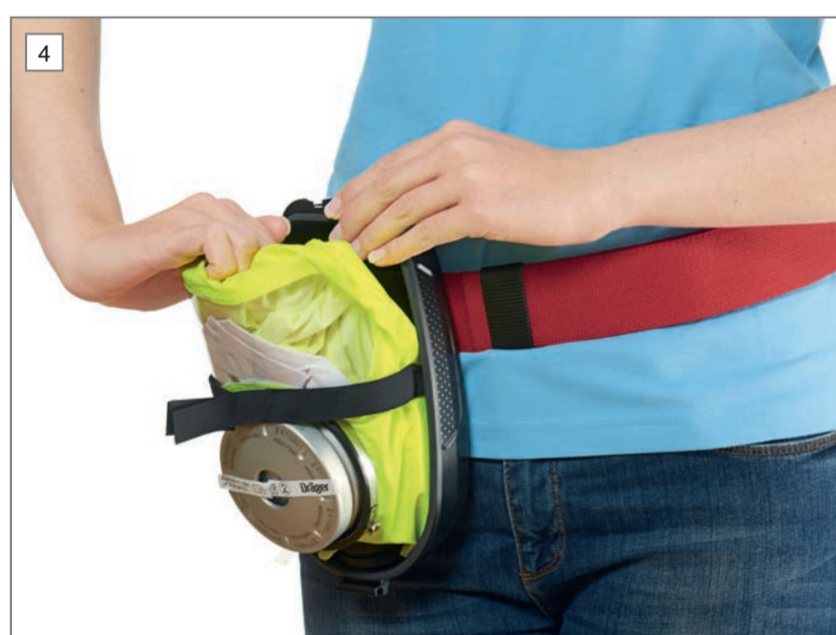
Remove the hood from the Hard Case. Pull the hood against the Velcro holder, it will automatically open. The second filter sealing plug will automatically be detached when the hood is removed.
