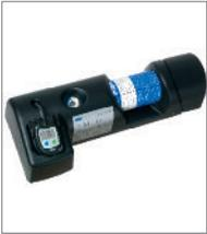
The Dräger Bump Test Station facilitates the performance of an everyday bump test, as the test is evaluated by the devices themselves and the test gas is automatically applied on insertion. In addition, most devices are able to automatically identify the station and switch to bump test mode without having to perform any manual activities.
