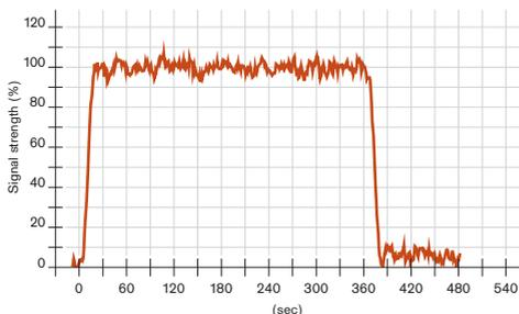
Linearity of H<sub>2</sub>S LC sensor
