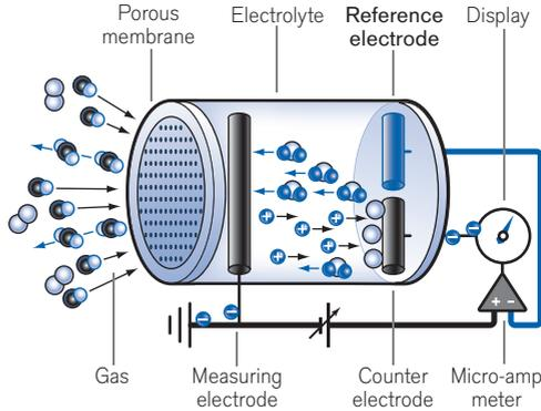
Chemical reaction at the measuring electrode
