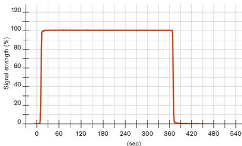
Linearity of NO sensor calibrated with 76 ppm NO
